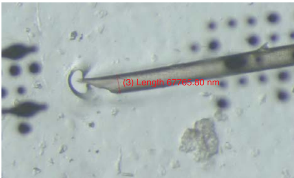
Figure 2. Hair measurement for diameter (denoted as length in the figure).
